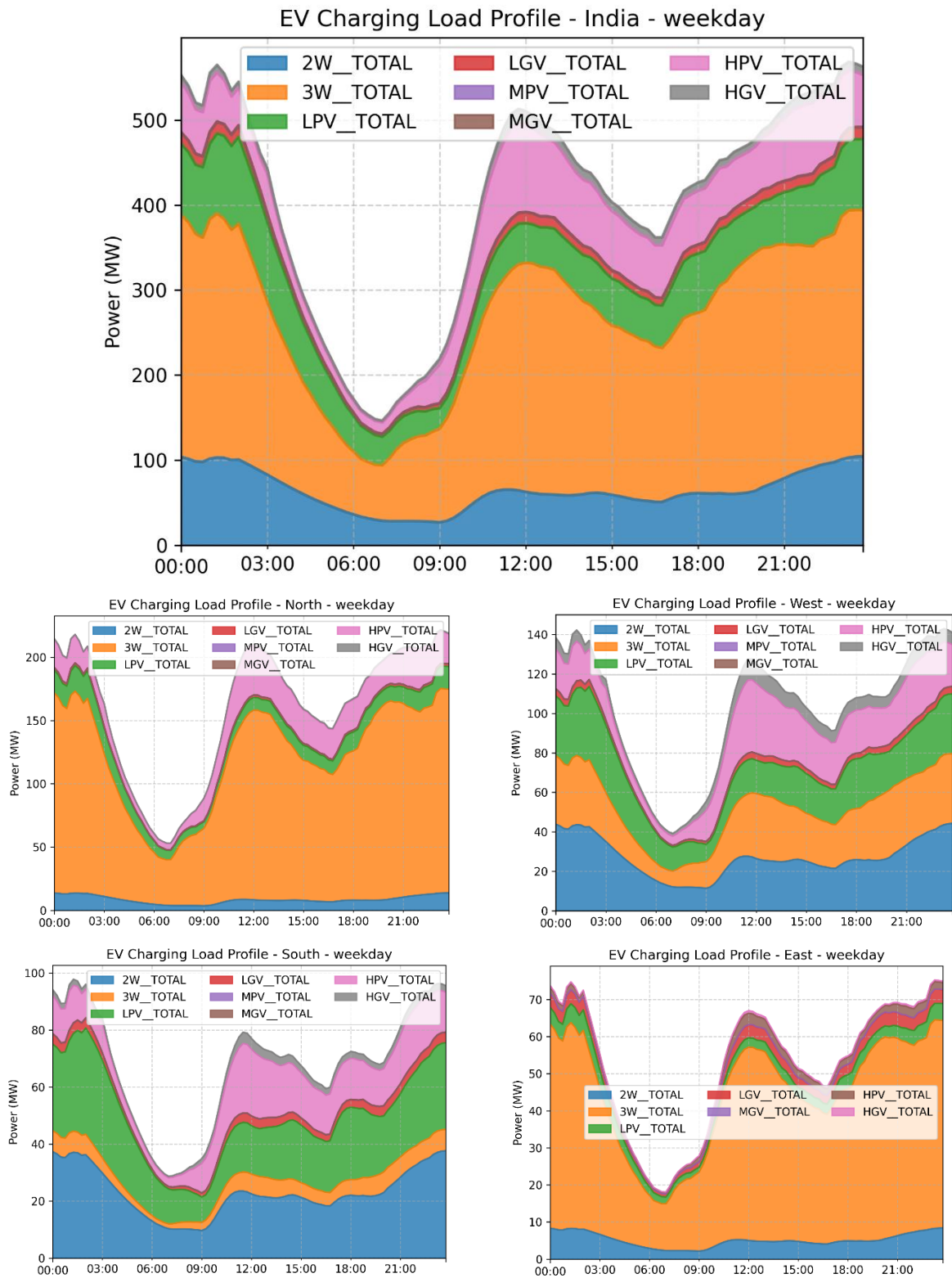
Figure 26: Weekday EV charging load profiles for India and regional grids, showing the aggregate charging power contribution of different vehicle categories across 24 hours.
